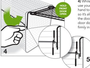
4) While holding the door open, use your finger with the opposite hand to turn the trigger rod up, so it's aligned with the groove of the door rod. Slowly move the door down, so the trigger rod rests firmly in the door rod grove.
