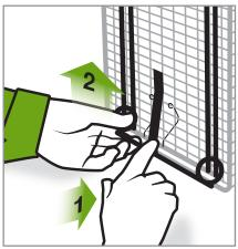
1) Push in front door lock and 2) slide ring rod up to the top of the door.
