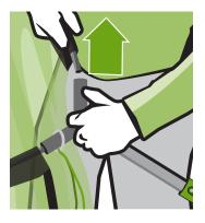
Unscrew non-ring side rod at "Y" and pulloff old net.
